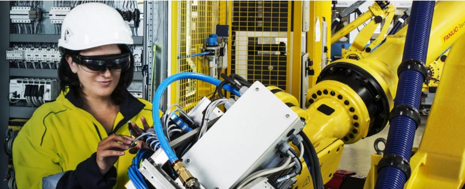
Dynacom Wearable Systems brings a customizable application environment to use cases where workers use monocular display smartglasses. The constrained viewing field of a single-eye display is used to flash alerts from data sources on the shop floor and provide access to simplified controls, including virtual keypads and control elements displayed on the palm of a user's hand and controllable with simple gestures.
