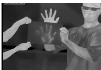
Residual heat detection
